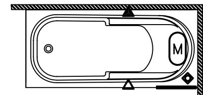
**M** Motor of single system (Hydro or Aero)
