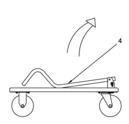
(3)Pull up the handlo 4 until the handle and cart is perpendicular
