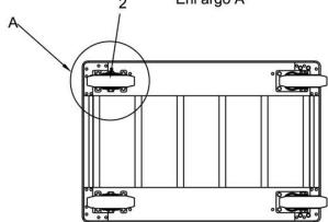
(2)Tum in reverse the cart, insert scrow 1 into mobile wheel 2(front wheel)& fixed wheel 3(rear wheel) and the screw hole in the bottom of the cart, then fasten it.
