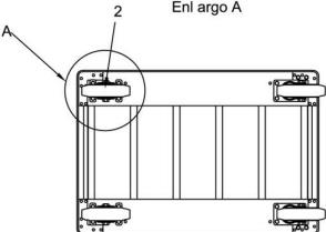
(2)Tum in reverse the cart, insert scrow 1 into mobile wheel 2(front wheel)& fixed wheel 3(rear wheel) and the screw hole in the bottom of the cart, then fasten it.
