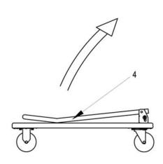
(3)Pull up the handlo 4 until the handle and cart is perpendicular
