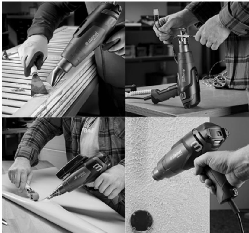
**Shaping PVC:** tiles, piping or ski boots can be softened and formed with hot air.
